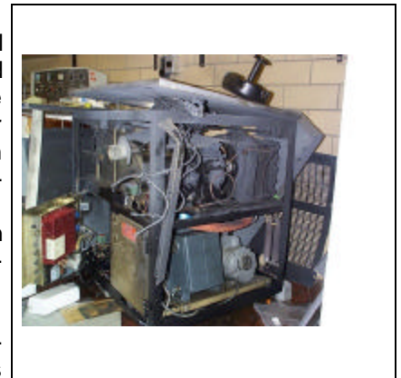
Remains from centrifuge explosion.
